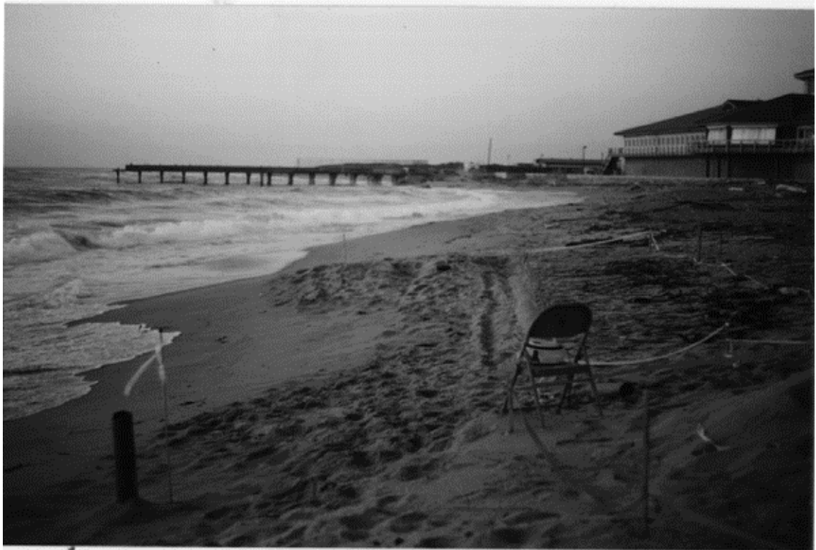
Figure 3: Tide at Moss-Landing beach. The seismic line was placed just below the high tide line, so at maximum tide the wave will wash the sand. The monitoring well (tube on the left) was placed 1.5m from the first geophone. The geophones were buried under the sand to reduce wave and wind noise. The geophone spacing was 20cm. At low tide the water table was 2m below the first geophone.
