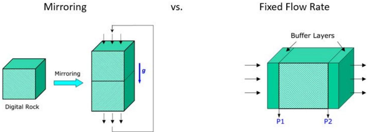
Figure B-2: (Left) constant forcing scheme with mirrored pore space geometry; (right) fixed flow rate scheme with a buffer zone of 15 pixels (Keehm and Bosl, 2003).
