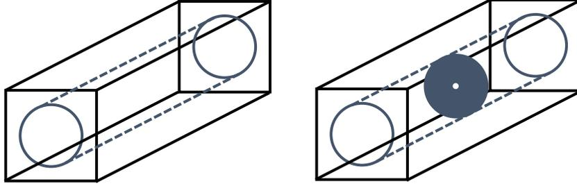
Figure 4-4: 3-D digital representation of a normal circular pipe and a circular pipe with a throat in the middle.
