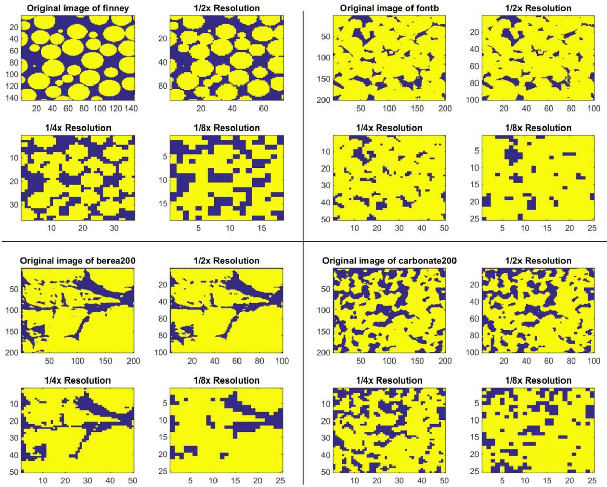
Figure B-9: Images of benchmark digital rock sample in 1x, 1/2x, 1/4x, 1/8x resolutions.
