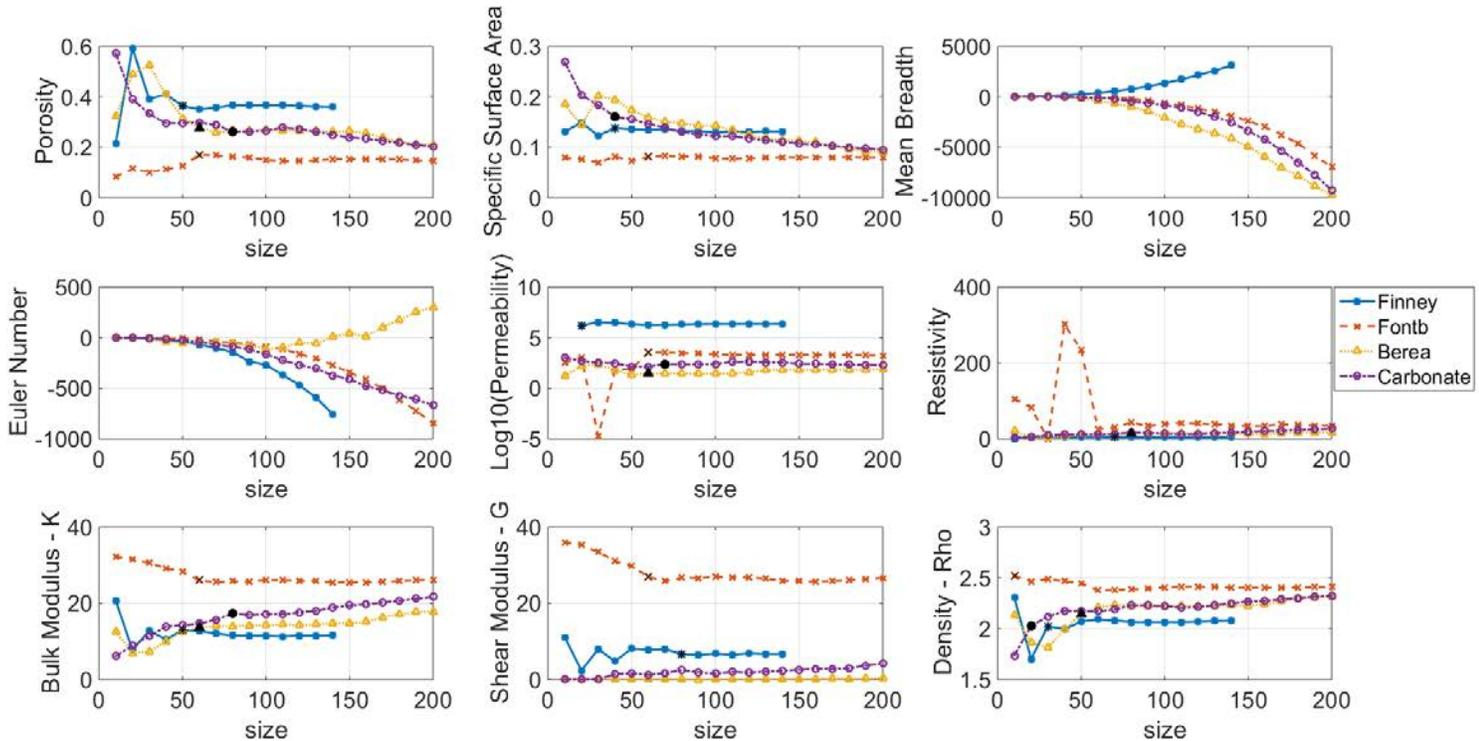
Figure B-8: Physical properties vs. sample size for all benchmark digital rock samples. The properties are (1) porosity, (2) specific surface area, (3) mean breadth, (4) Euler number, (5) permeability on a log 10 scale, (6) resistivity, (7) bulk modulus, (8) shear modulus, and (9) density.
