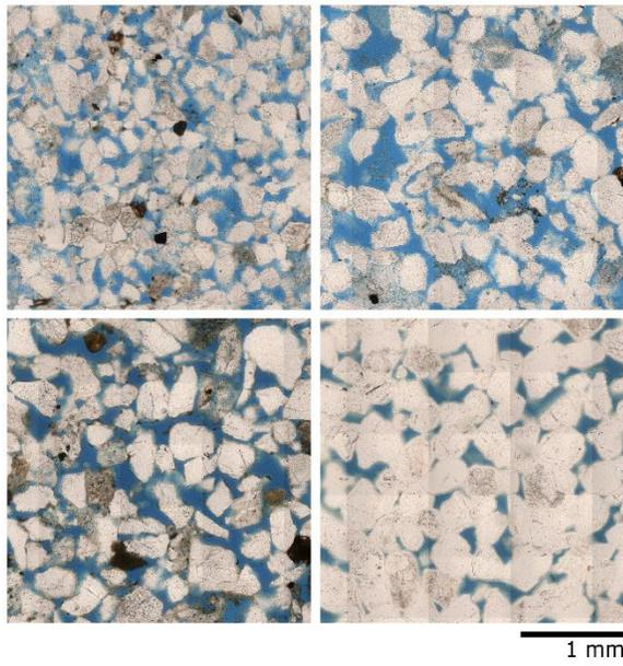
Figure 8-5: Cropped 2-D thin sections from B1, B5, CG1, and FB24 from top-left to bottom-right.
