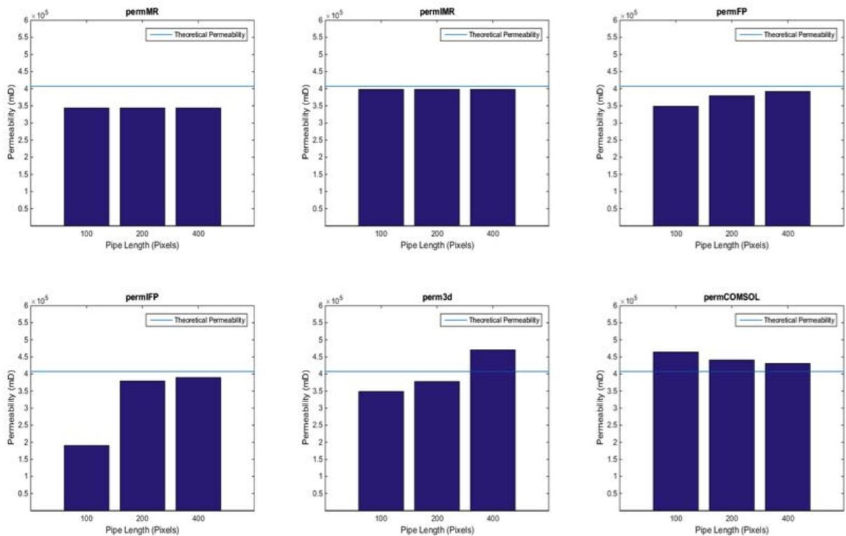
Figure B-3: Comparison of permeability predictions in a circular pipe from five different versions of the Lattice Boltzmann program and the COMSOL finite element program. The blue line in each graph represents the theoretical permeability value. In each graph, the length of the pipe is 100, 200, or 400 pixels.
