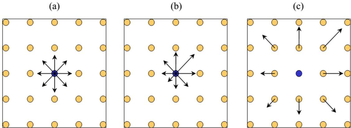
Figure B-1: Steps of the Lattice-Boltzmann algorithm: (a) initial state of the density distribution, (b) collision step, (c) propagation step (Keehm and Bosl, 2003).
