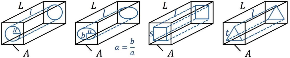
Figure 4-1: 3-D digital representations of a circular pipe, an elliptical pipe with aspect ratio 0.7, a square pipe, and an equilateral triangular pipe.
