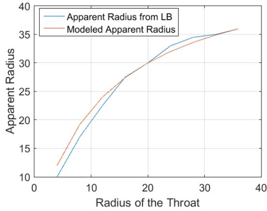
Figure 4-5: Comparison of the apparent radius calculated from Lattice Boltzmann simulations to that from the apparent radius model. The x axis represents the radius of the throat, which ranges from 4 to 36 pixels.
