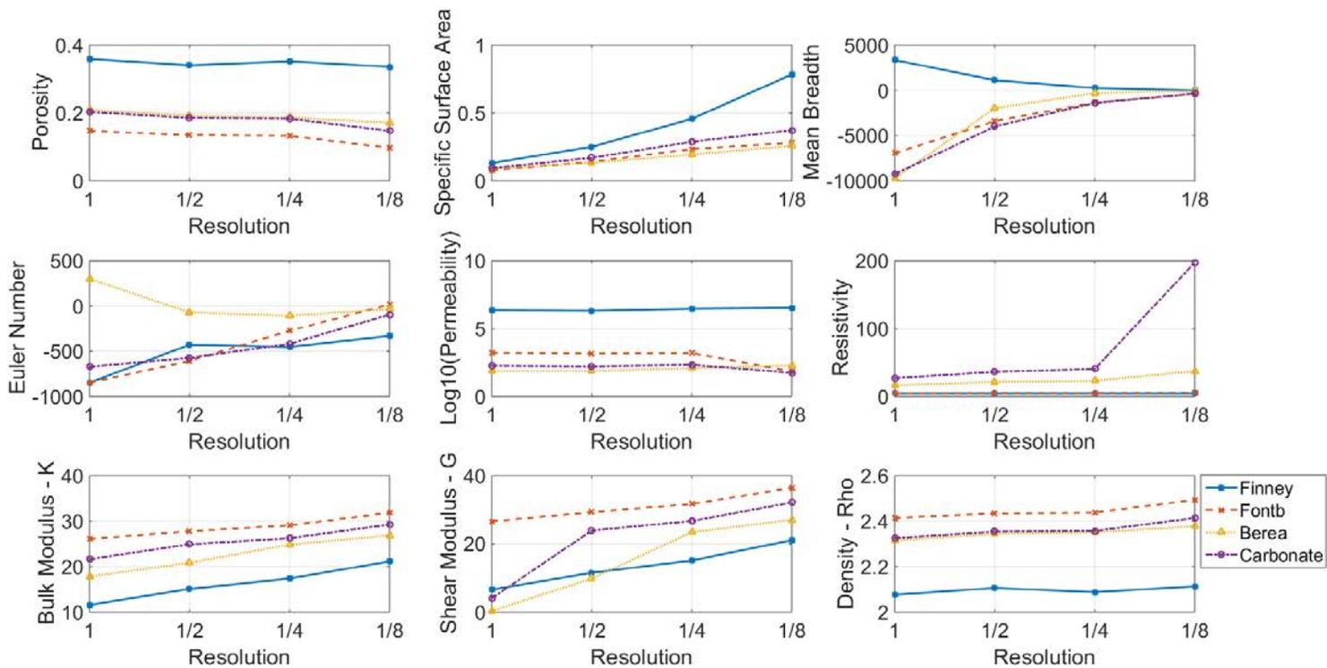
Figure B-10: Physical properties vs. resolution of each sample. The properties are (1) porosity, (2) specific surface area, (3) mean breadth, (4) Euler number, (5) permeability in log 10 scale, (6) resistivity, (7) bulk modulus, (8) shear modulus, and (9) density.
