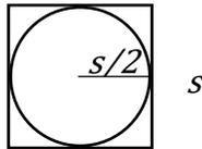
Figure 4-3: Cross-section of a square pipe of side  $s$ . The hydraulic radius is  $s/2$  which is exactly the radius of a circle inscribed in the square.
