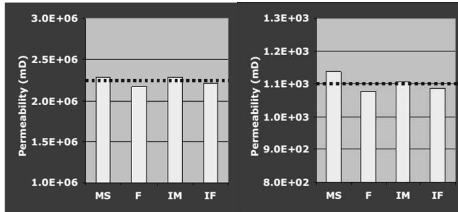
Figure B-4: Calculated Permeability (mD) of Finney Pack (left) and Fontainebleau Sandstone (right) for four different versions of the Lattice Boltzmann algorithm (MS = MR, F = FP, IM = IMR, IF = IFP) from (Keehm and Bosl, 2003).
