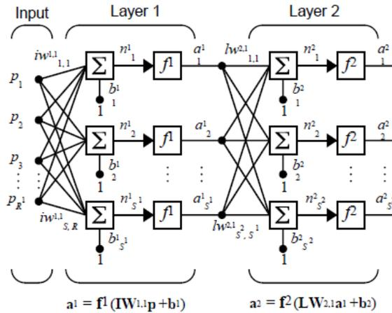
Figure 7-4: Example of the network architecture (Demuth, 2002).
