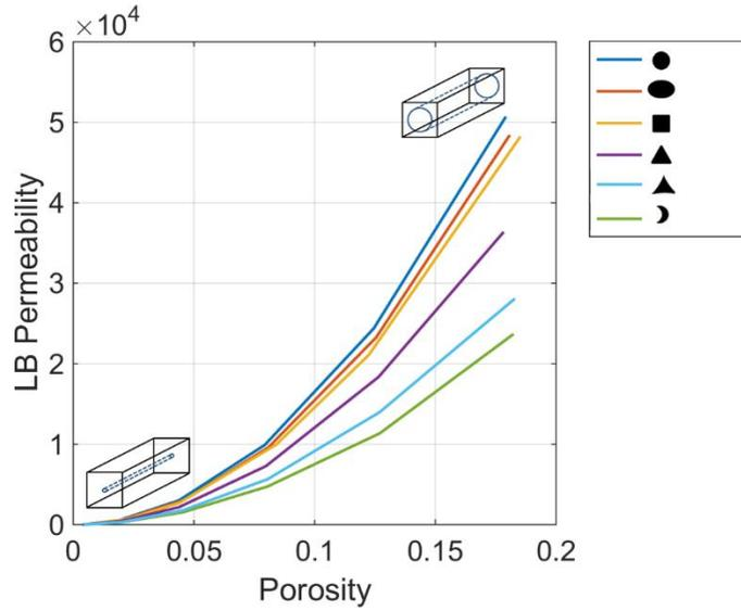
Figure 4-2: For all pipes with the same porosity, a circular pipe has the highest permeability. The ratio of the permeability of any cross-section to that of a circular cross-section can be found using the apparent radius concept. In this case, the permeability is calculated using Lattice-Boltzman flow simulation.
