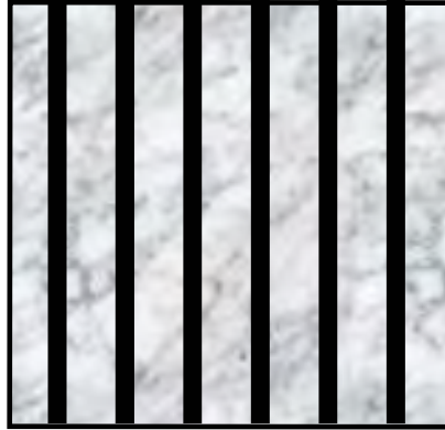
Figure 2.2: Graphical representation of fractures using the linear-slip model with infinitely long planes of weaknesses.
