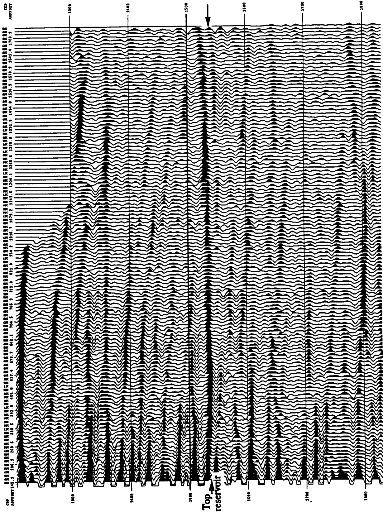
Figure 5.58: Seismic CDP supergather within the vicinity of well 31/2-5 (approximately CDP 355); close-up on the reservoir zone.
