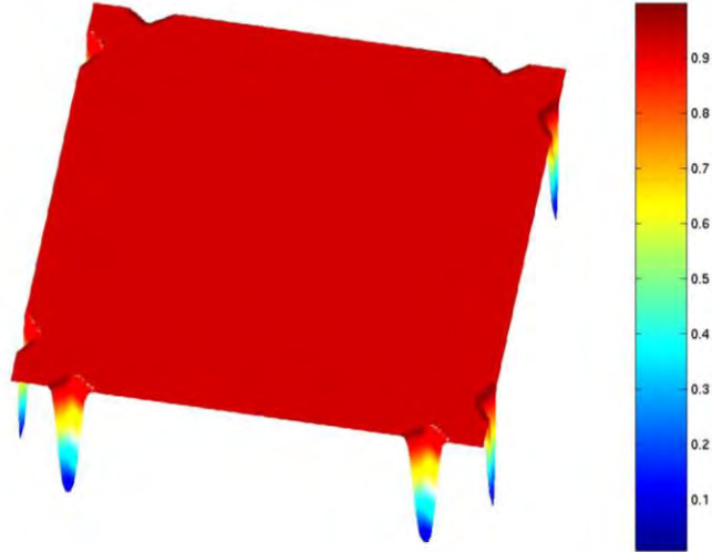
Figure 8.8. Crossings taper at the positions of the intersections for an aliased frequency of 25 Hz.
