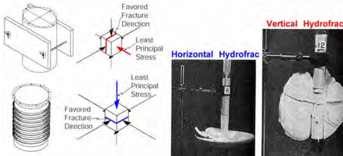
Figure 4.15. Hydraulic fractures always propagate perpendicular to the orientation of the least principal stress.
