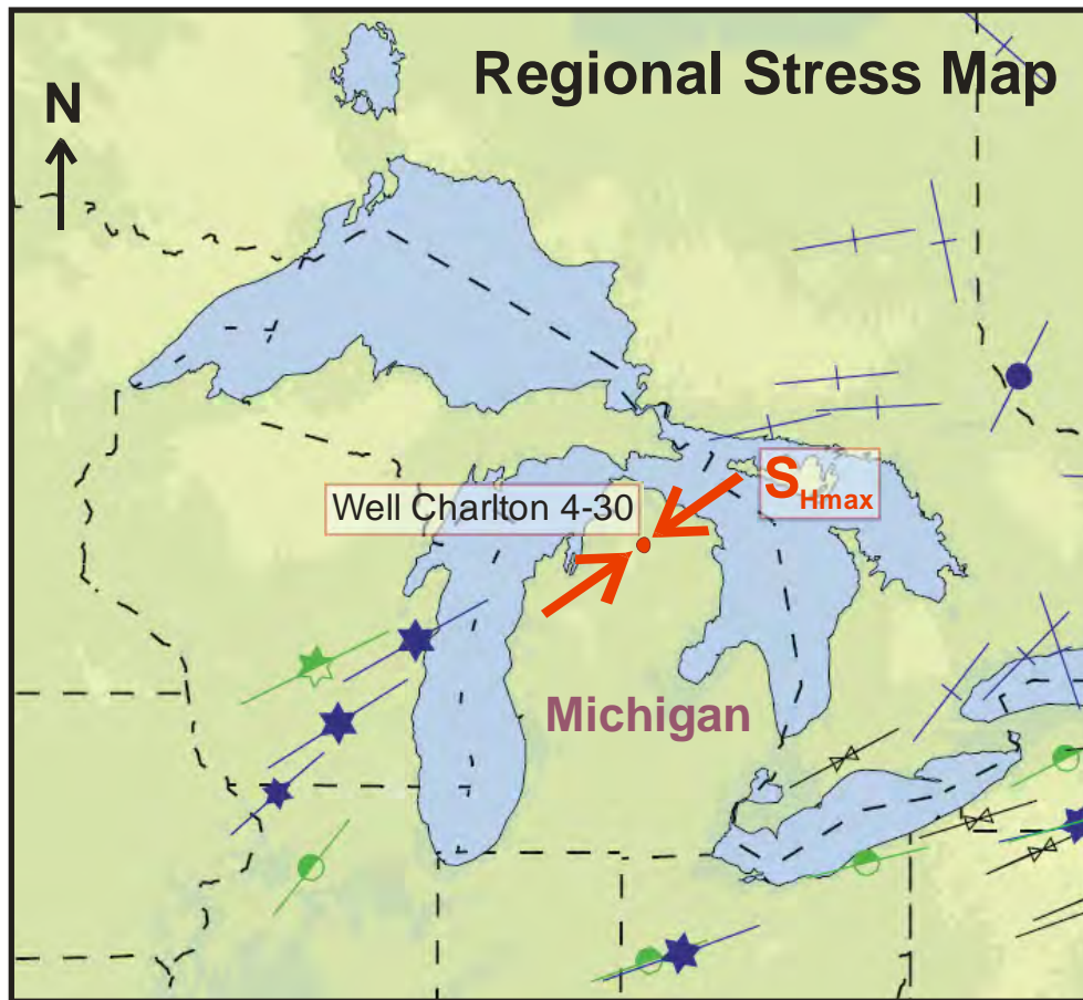
Figure 6.6: Regional Stress map modified from Reinecker et al, (2005). The red arrow indicates the S_{Hmax} direction determined in the present study.
