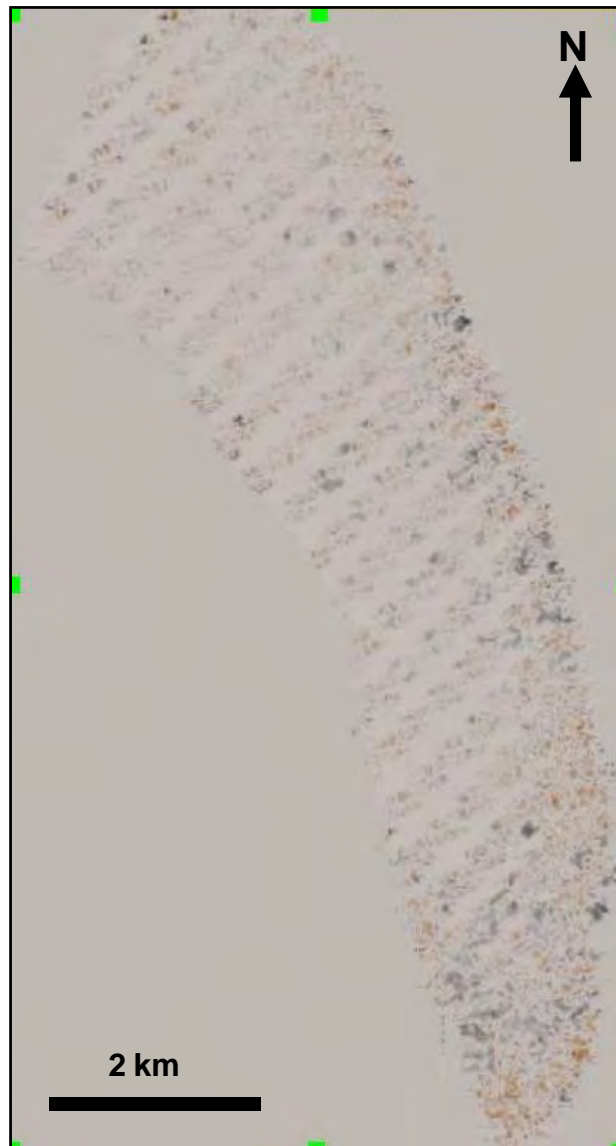
Figure 5.41: Amplitude time-slice showing the acquisition pattern of the Teapot Dome 3D seismic volume.
