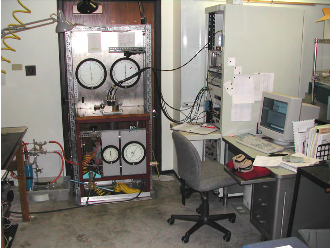
Figure 2.1: The experimental apparatus. The electrical leads for the strain gauges and ultrasonic transducers can be seen to run from the top end cap of the vessel at the center of the pressure vessel stand (center left) to the electronics located in the stand on the right. The computer used to record the ultrasonic signals is shown on the desk. The pore pressure degassing system lies on the floor to the left of the vessel stand.
